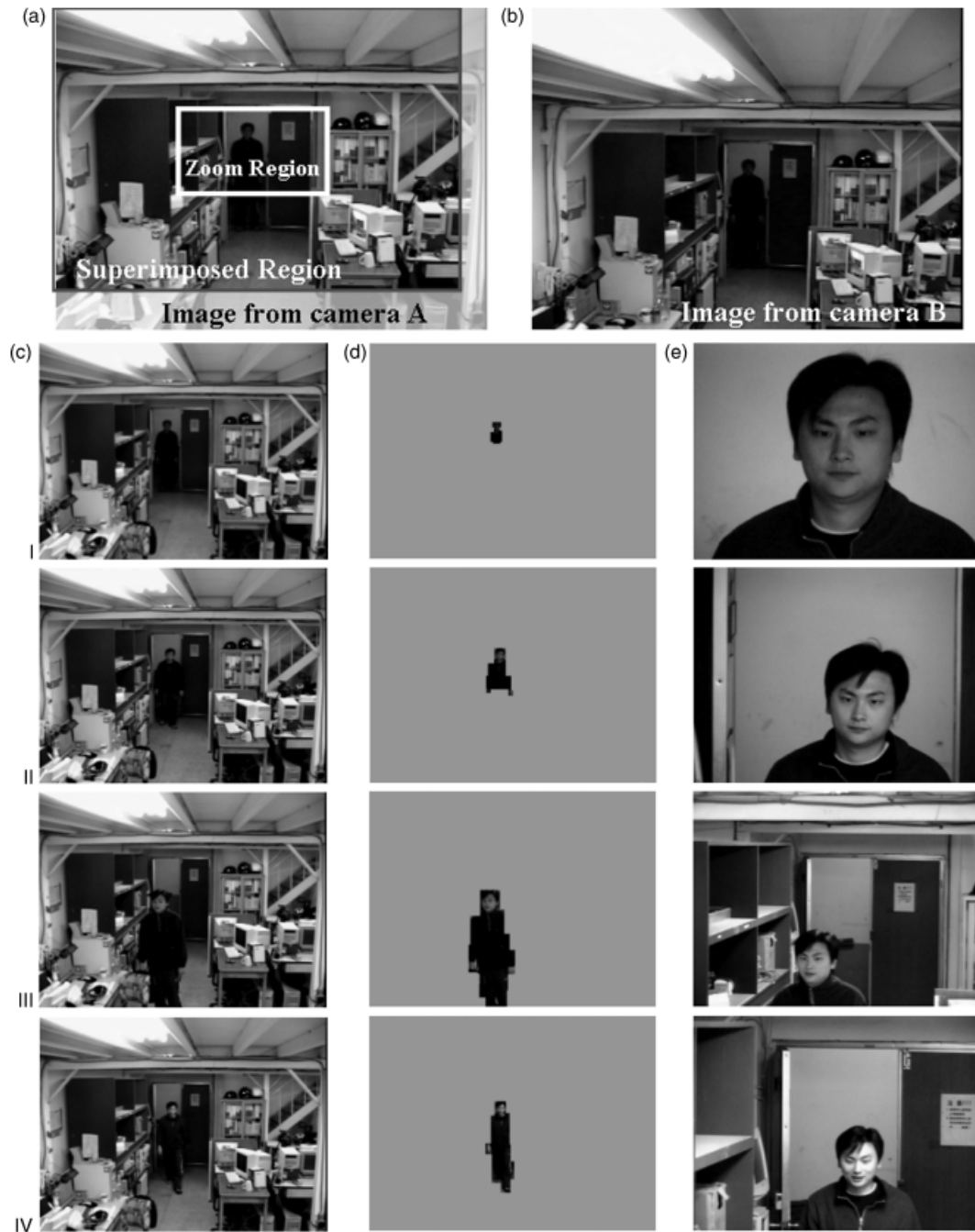
FIG. 6—Example: (a) an image from camera A and the superimposed region obtained by the camera position translation analysis process; (b) an image from camera B; (c) some image sequences from camera A; (d) the moving-object detection results; (e) some image sequences from camera B.
